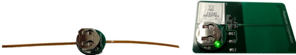
The Radio Boards correctly connected to the Battery Recharging Boards
