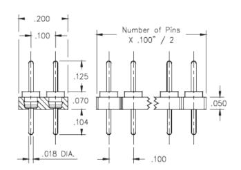
**Description:** Interconnect Header Low Profile Solder Tail Header .018" (0,46mm) Pin Head Double Row Through Hole Plating Code: 10 Shell Plating: 10 µ" Gold over 100 µ" Nickel
