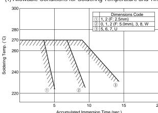
Perform soldering within tolerance range (shaded portion).
