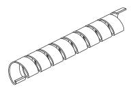
Spiral Wrap is an ideal covering used to bundle and protect tubing, wires, and other types of conductors. Spiral wrap can be used on virtually any item with a diameter of 1/16" to 7". Polyethylene Natural Spiral Wrap is a lightweight low cost material that is good for general indoor applications. Polyethylene is not affected by ordinary solvents and is resistant to abrasion.
