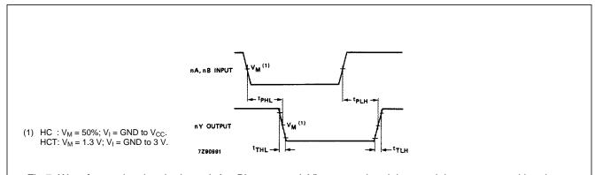
Fig.7 Waveforms showing the input (nA, nB) to output (nY) propagation delays and the output transition times.
