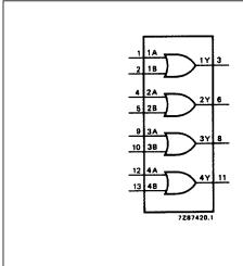
Fig.4 Functional diagram.
