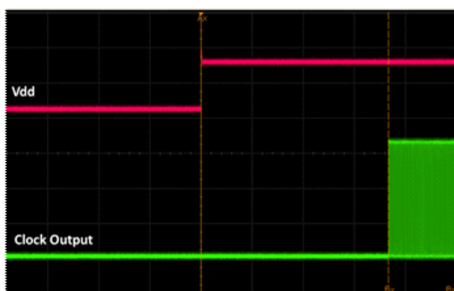
Figure 17. Startup Waveform vs. Vdd
