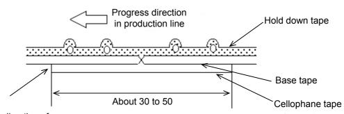
No lifting for the direction of progressing
