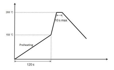
\* Recommended Temperature Profile for Reflow Soldering
