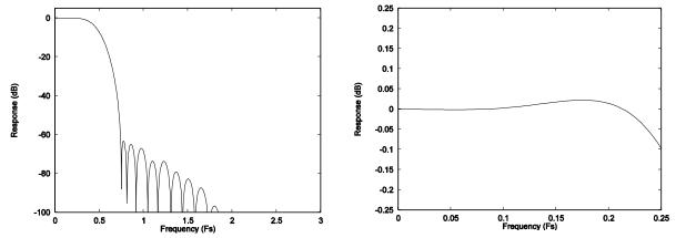
Figure 35 ADC Digital Filter Frequency Response – Type 2 Figure 36 ADC Digital Filter Ripple – Type 3
