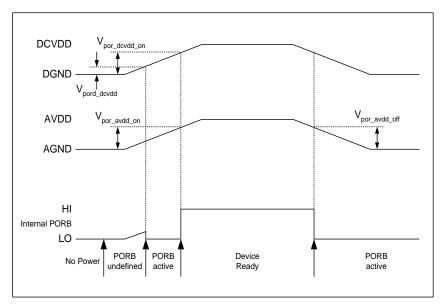
Figure 7 Typical Power-Up Sequence
