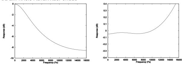
Figure 37 De-emphasis Frequency Response (32kHz)
