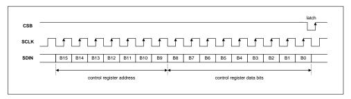
Figure 19 3-Wire Serial Control Interface
