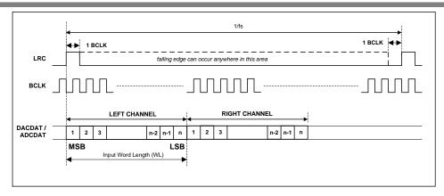
Figure 17 DSP/PCM Mode Audio Interface (mode B, LRP=0, Slave)
