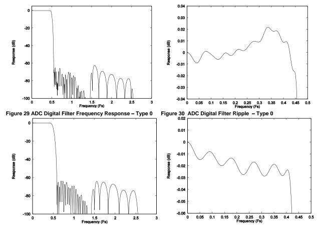
Figure 31 ADC Digital Filter Frequency Response - Type 1 Figure 32 ADC Digital Filter Ripple - Type 1
