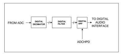
Figure 8 ADC Digital Filter
