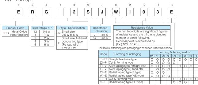
The above example 2 shows a small metal oxide film resistor, 2 W power rating, resistance value of 10 kΩ, tolerance ±5 %, and package of radial taping
