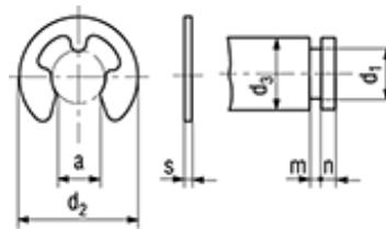
**BN 809****Circlips for shafts**
