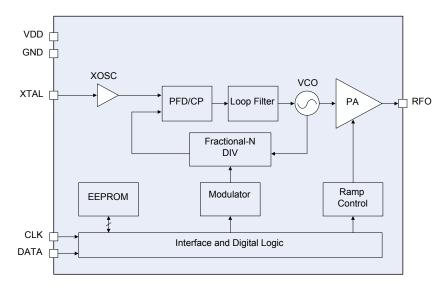
Figure 11. RFM119/S Functional Block Diagram
