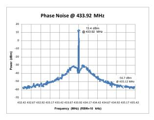
Figure 3. Phase Noise,  $F_{RF}$  = 433.92 MHz,  $P_{OUT}$  = +13 dBm, Unmodulated
