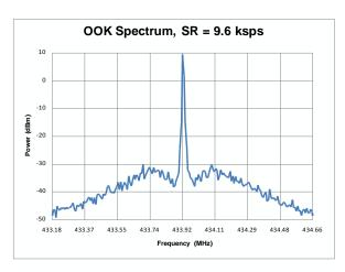
Figure 5. OOK Spectrum, SR = 9.6 ksps,  $P_{\text{OUT}} = +10 \text{ dBm}, t_{\text{RAMP}} = 32 \text{ us}$
