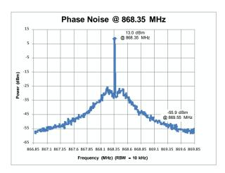
Figure 4. Phase Noise,  $F_{RF}$  = 868.35 MHz,  $P_{OUT}$  = +13 dBm, Unmodulated
