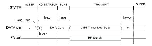
Figure 16. Transmission Enabled by DATA Pin Rising Edge
