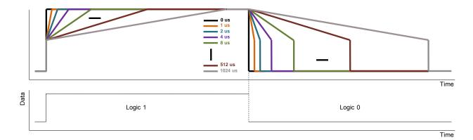
Figure 13. PA Ramping Time
