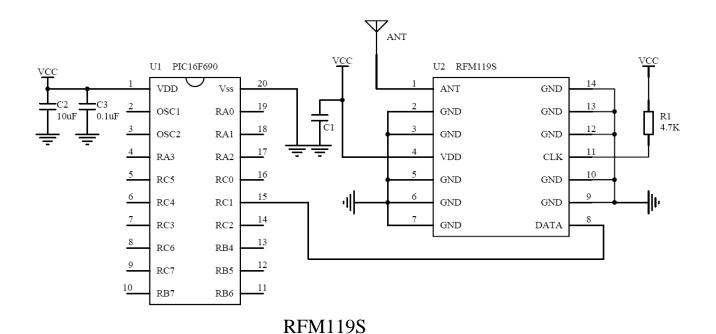
Figure 9: Typical Application Schematic
