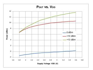
Figure 8. Output Power vs. Supply Voltages, F<sub>RF</sub> = 433.92 MHz
