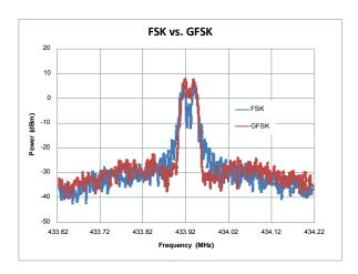
Figure 6. FSK/GFSK Spectrum,  $SR = 9.6 \text{ ksps}, F_{DEV} = 15 \text{ kHz}$
