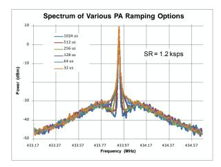
Figure 7. Spectrum of PA Ramping, SR = 1.2 ksps, P<sub>OUT</sub> = +10 dBm
