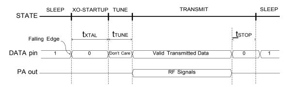
Figure 17. Transmission Enabled by DATA Pin Falling Edge
