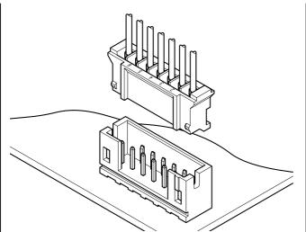
This is a thin, low-profile 2.0mm pitch connector 8.0mm in height after mounting and 4.5mm in width. It is designed to meet the demand for high-density connection of internal wires to printed circuit boards. It is compact, highly reliable and low in cost.
