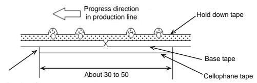
No lifting for the direction of progressing
