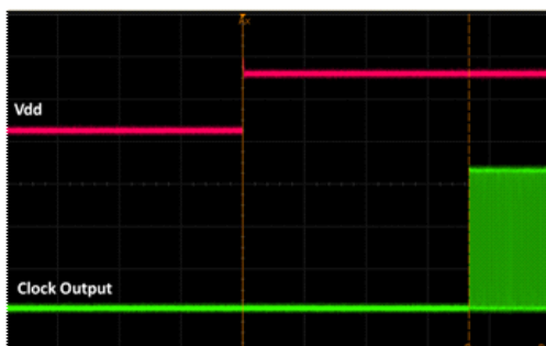
Figure 17. Startup Waveform vs. Vdd
