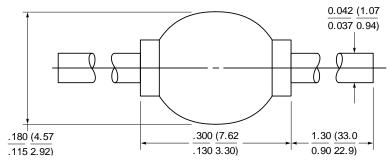
Note: The cathode side is marked with a dark colored band on one side of the diode body.
