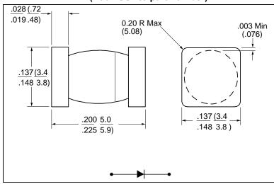
Note: The cathode side is marked on body with a dark band.
