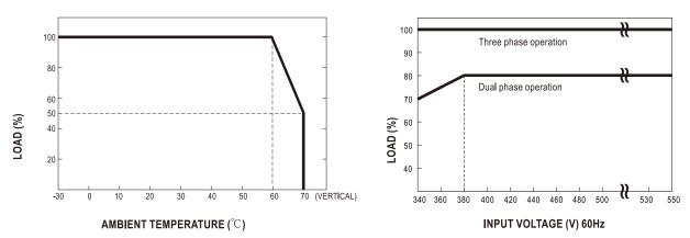
Note: When the dual phase input voltage is between 340~380 Vac and ambient temperature is between -10°C ~-30°C, the power supply may experience hiccup at cold start. The power supply will start up normally after 5~10 seconds.
