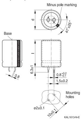
Snap-in terminals, length  $(6.3 \pm 1)$  mm. Also available in a shorter version with a length of (4.5 - 1) mm. PET insulation is marked with "PET" on the sleeve. Safety vent on the base.
