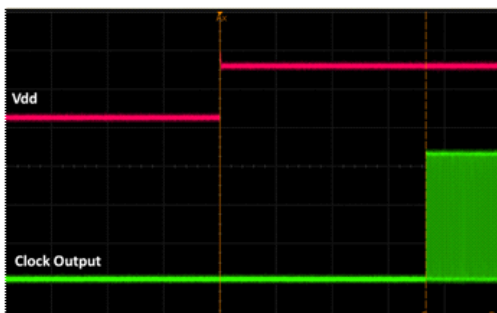
Figure 17. Startup Waveform vs. Vdd
