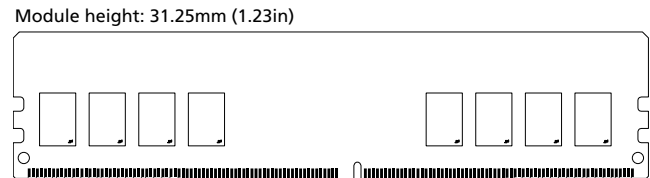
Figure 2: 288-Pin UDIMM (MO-309 R/C A2)
