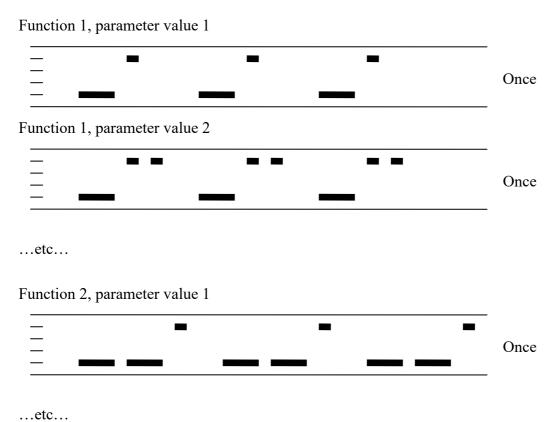
If the throttle stick is moved to zero during one of the above sequences, the parameter value of that function is selected and stored. And you will hear this sound:
