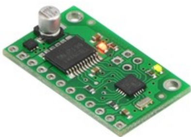
Pololu qik 2s9v1 dual serial motor controller.
