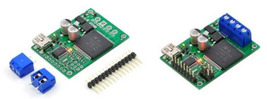
The jrk ships with a straight 0.1" breakaway male header strip and two 5mm, 2-pin terminal blocks. To provide maximum flexibility, none of these parts are soldered to the board.
