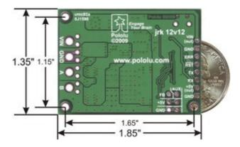
The jrk 12v12 is a versatile, general-purpose motor controller that supports a variety of interfaces, including USB. The 6 V to 16 V operating range and high continuous output current of 12 A (30 A peak) allow this board to control many medium-sized DC brushed motors. Analog voltage and tachometer (frequency) feedback options allow quick implementation of closed-loop servo systems, and a free configuration utility (for Windows) allows easy calibration and configuration through the USB port.
