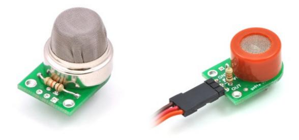
Pololu MQ gas sensor carrier with sensitivitysetting resistor soldered in the horizontal orientation.
