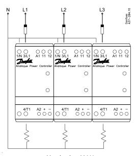
Max. load at: 230 V 3 x ACI 30-1 20.7 kW 3 x ACI 50-1 34.5 kW Three phase with single-phase contactor ECI-1 as slave Only burst firing mode
