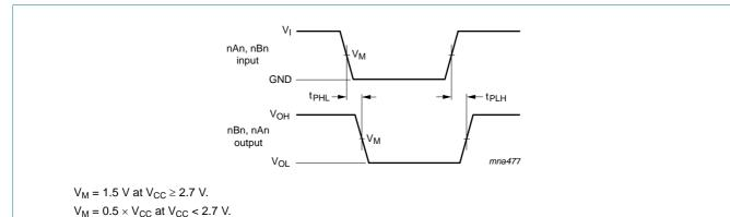
V<sub>OL</sub> and V<sub>OH</sub> are typical output voltage levels that occur with the output load. Fig 5. The input (nAn, nBn) to outputs (nBn, nAn) propagation delays
