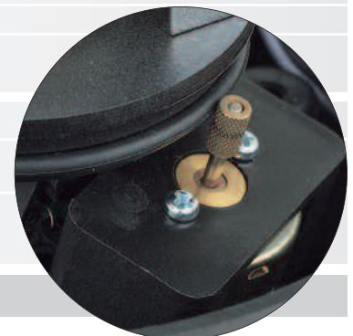
Low wear wheel and disc drive
