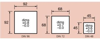
DIN 48 can be slot mounted using the standard fixing clip. DIN 72 & DIN 96 can be supplied with special fixing clips for slot mounting. Slot dimensions available on request.
