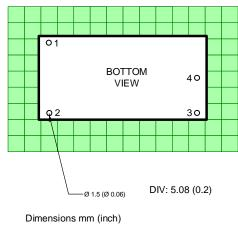
Dimensions mm (inch) Case Tolerance  $\pm 0.50$  ( $\pm 0.02$ ) Pin Diameter 1.0  $\pm 0.10$  (0.04  $\pm 0.004$ ) Pin Pitch Tolerance  $\pm 0.35$  ( $\pm 0.014$ )
