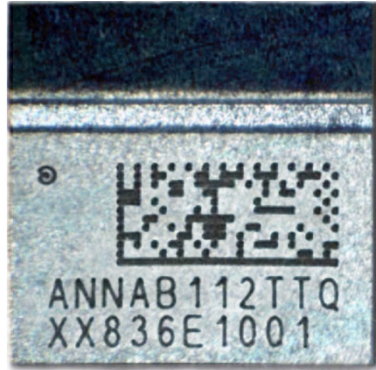
Figure 10: Product marking on the ANNA-B112 module
