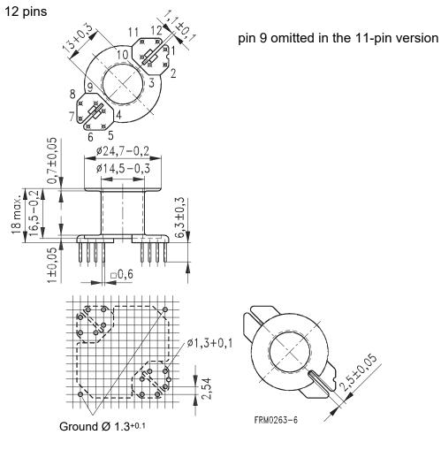
Hole arrangement View in mounting direction
