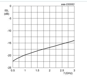
Diode zero-biased and inserted in series with a 50  $\Omega$  strip line circuit; T\_{amb} = 25  $^{\circ}\text{C}$
