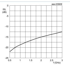
Diode zero-biased and inserted in series with a 50  $\Omega$  strip line circuit and biased via the analyzer T-network; T<sub>amb</sub> = 25 °C; f = 100 MHz
