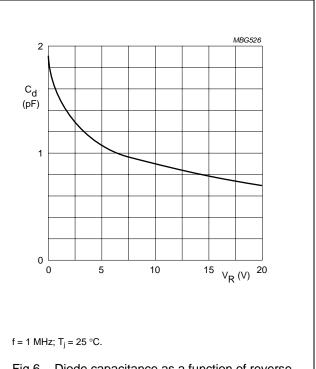
Fig.6 Diode capacitance as a function of reverse voltage; per diode; typical values.
