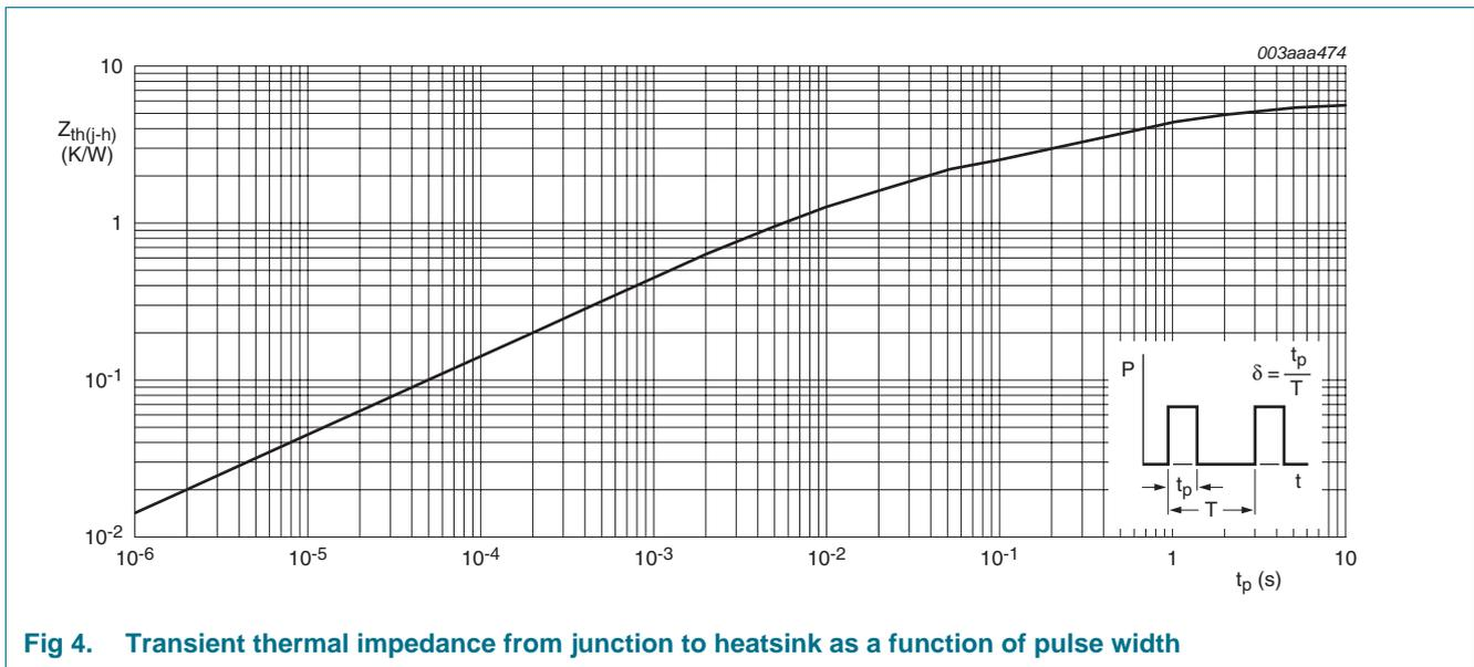
Fig 4. Transient thermal impedance from junction to heatsink as a function of pulse width
