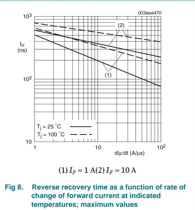
Fig 8. Reverse recovery time as a function of rate of change of forward current at indicated temperatures; maximum values
