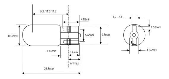
**Filament construction C-2V**
