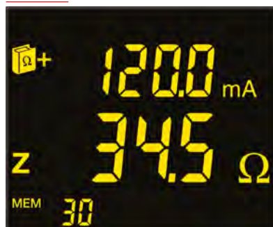
Screen 1: Impedance and leakage current
