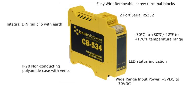
Booster for RS232 signal can extend cable length. Works with a wide voltage swing and outputs -11V to +11V signal making it suitable for legacy and non-conforming RS232 equipment. Provides isolation between two RS232 devices. This product doesn't require any software, simply connect using the easy-wire numbered terminal blocks.
