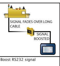
RS232 signal can degrade over long cable runs. The CB-534 boosts the RS232 signal enabling additional distance between connections.
