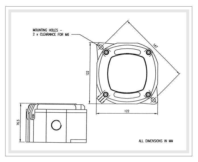
**INSTALLATION INSTRUCTIONS:** The installer must ensure that the enclosure chosen is suitable for the field of application. Which means that the marking on the certification label must correspond to the classification given to the Ex area.
