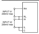
To determine the ratio between two voltages apply the inputs as shown.
