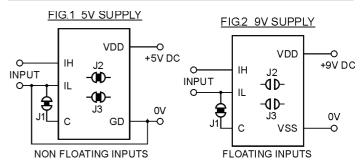
For 9V operation it is recommended to power from a 9V battery. The inputs are intended to float with respect to the supply but if they do not float they must be no closer than 1.5V from either VDD or VSS (VDD-1.5V and VSS+1.5V) see the circuits for non-floating inputs below.
