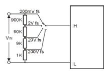
For multi-range, use a 2 pole, 4 way rotary switch. 1 pole for range select and the other to connect the appropriate decimal point to XBP.
