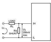
Shunt resistance Rs =  $\frac{Vs}{IIN} \Omega$
