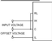
To achieve a zero display reading for a non-zero voltage input, apply the offset voltage between C and IL.
