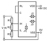
Using the formulae choose resistors to ensure the analogue inputs are no closer than 1.5V from either VDD or VSS (VDD-1.5V or VSS+1.5V)
