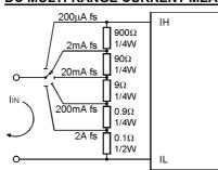
For multi-range, use, a 2 pole, 5 way rotary switch. 1 pole for range select and the other to connect the appropriate decimal point to XBP
