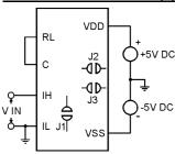
Where a single 5V supply is not suitable but you must connect your input signal ground to the module supply ground then either of the two non-floating input circuits can be used. Note that the module is set in 9V supply mode BUT jumper J1 is left open.
