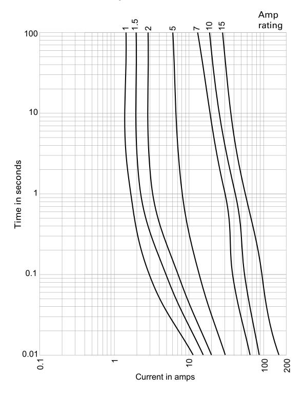
Non-rejecting, fast-acting GLR fuse and HLR in-line fuse holders
