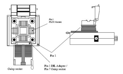
Please note: For converting 32-pin DIL to 32-pin PLCC, a different adapter is required!
