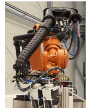
igus® chainflex® cables in triflex® R e-chain® for 6-axis robots
