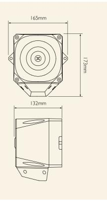
The Asserta Midi Sounder Beacon is a versatile and rugged audio-visual alarm designed for industrial environments or areas where there is a requirement for a physically robust and well-protected unit. A range of supply options permit use with a wide range of fire and process systems.
