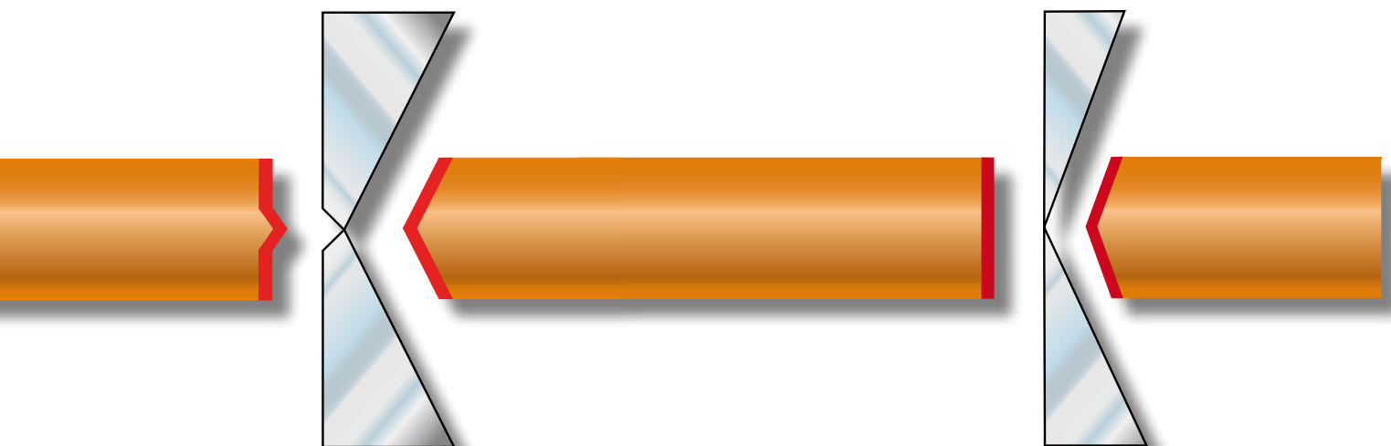
THE FLUSH CUT
