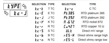
Select the input type that corresponds to the input sensor. For RTD types, check the RTD Input Jumper for matching selection. For sensor verification and testing, use the direct readout modes.
