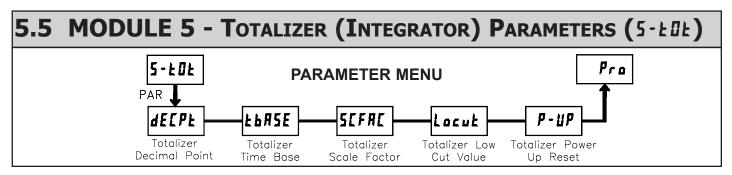
The totalizer accumulates (integrates) the Input Display value using one of two modes. The first is using a time base. This can be used to compute a timetemperature product. The second is through a user input or function key programmed for Batch (one time add on demand). This can be used to provide a readout of temperature integration, useful in curing and sterilization applications. If the Totalizer is not needed, its display can be locked-out and this module can be skipped during programming.
