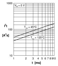
Fig. 3 I<sup>2</sup>t versus time (1-10 ms)
