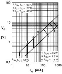
Fig. 4 Gate trigger characteristics
