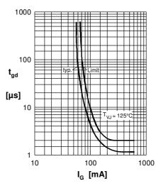
Fig. 5 Gate controlled delay time
