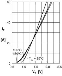
Fig. 1 Forward characteristics
