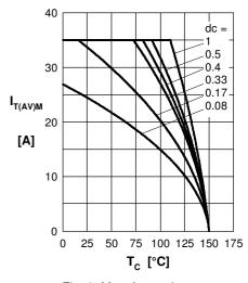
Fig. 6 Max. forward current at case temperature
