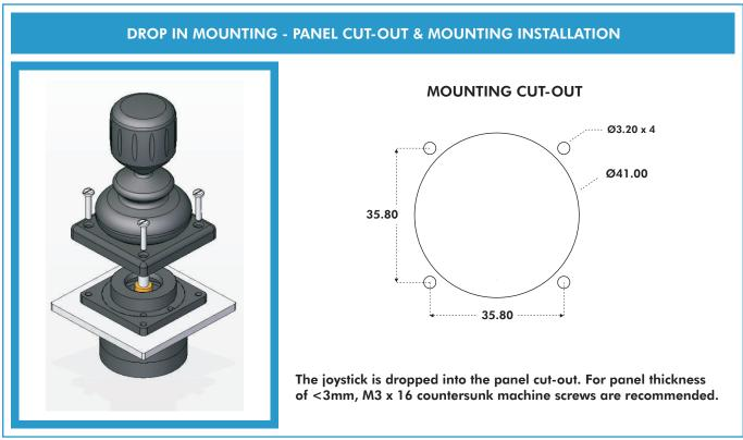
Note: The dimensions shown are for a generic 9000 Series with the third axis R type handle. For specific dimensions of this or any other configuration please refer to Apem.
