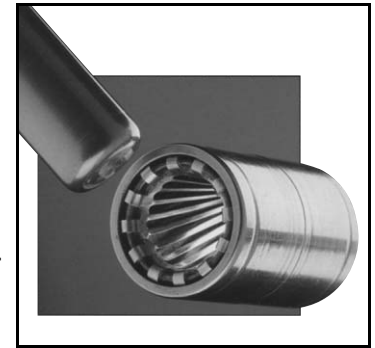
The RADSOK design - socket cylinder within female contact has twisted hyperbolic grid. Provides higher amperage capabilities with low insertion force and low temperature rise.
