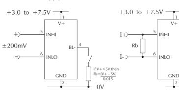
Measuring a current from a circuit which is floating with respect to the DPM's supply, i.e. the current and the meter's power supply are isolated from each other. Ensure solder link LCOM is closed.
